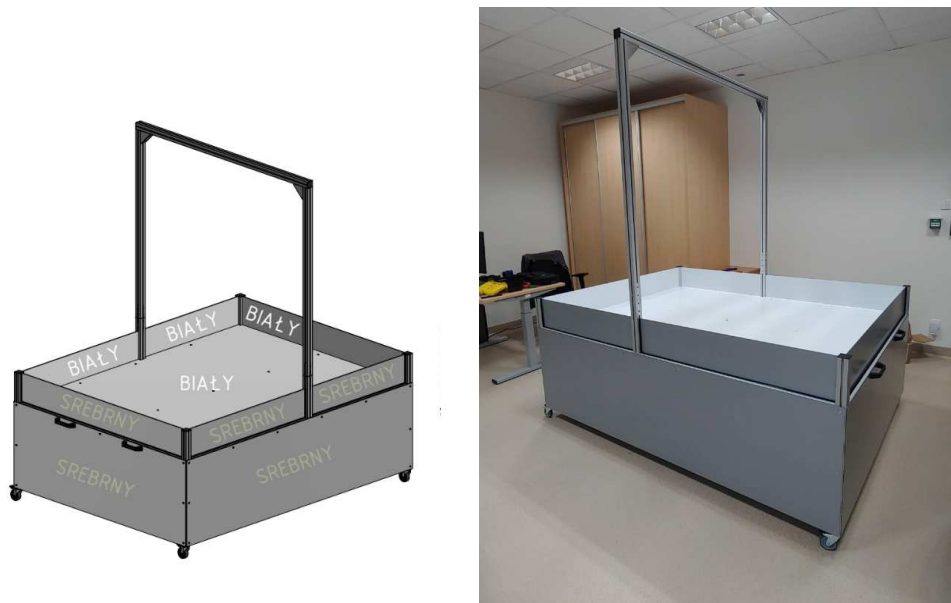
Figure 9. Visualization and realisation of the controlled environment for the empathetic robot swarm – arena.
