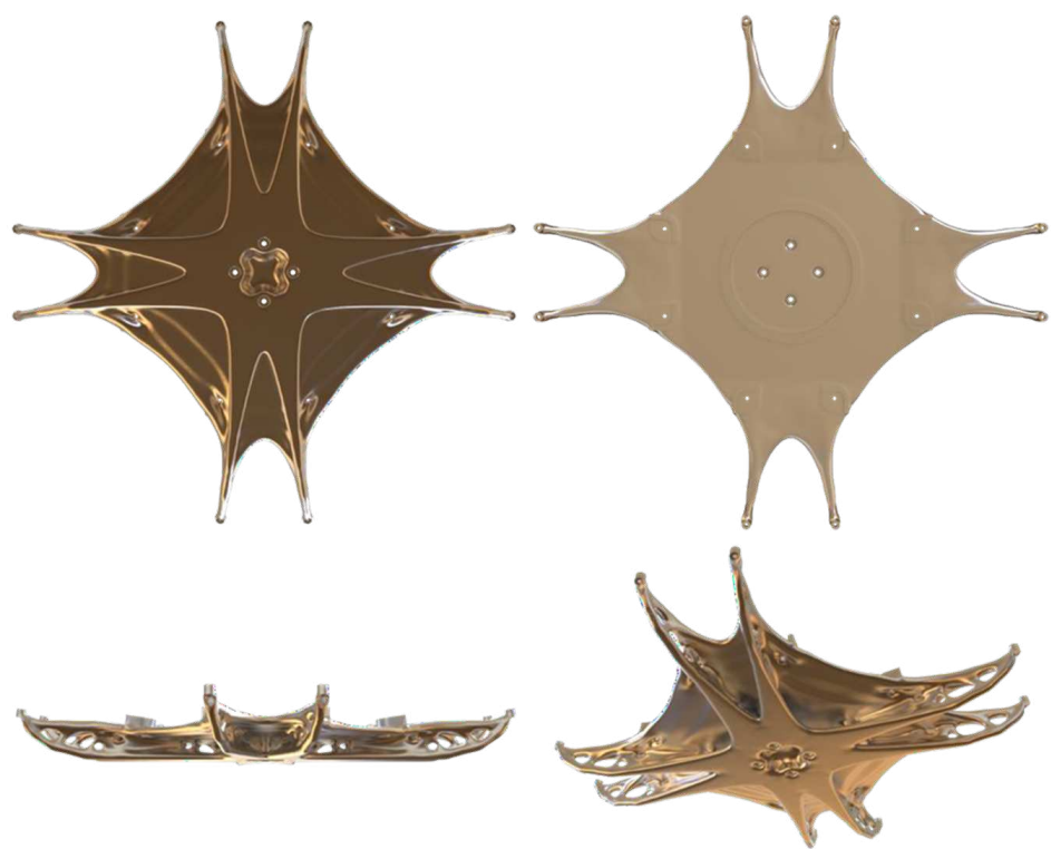
Figure 10. Topology optimized concept geometry for a 5 kg target mass and short envelope.
