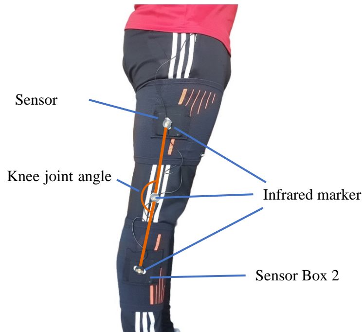
Figure 9. Sensor Boxes attached with bandages to the thigh and shank of the right leg. Additionally, three infrared markers for an optical MAS are attached to the leg. They form a triangle that covers the angle \alpha of the knee joint.
