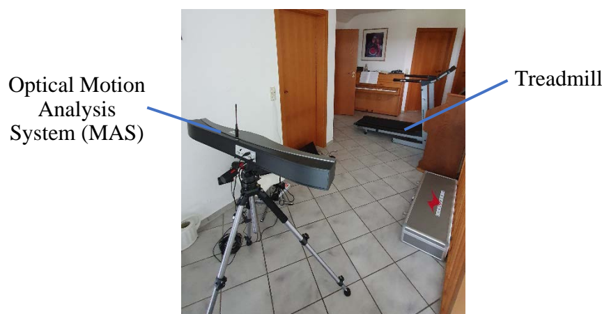
Figure 8. Treadmill Test setup with optical MAS positioned three meters away from the treadmill.
