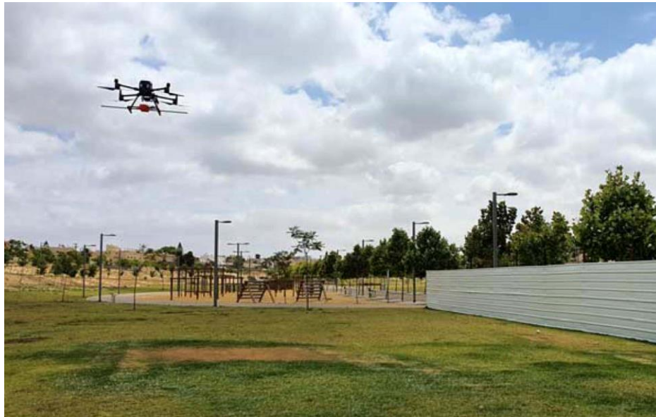
Figure 3. A DJI M-300 drone with a GPR 150 MHz dipole antenna at the bottom provides subsurface sensing capabilities up to 15 m below the surface. The Sky-Hub computer, which is positioned on the right side, is responsible for controlling automatic flight operations. At the front of the drone, a small radar (altimeter) measures the distance from the ground, maintaining a constant flight altitude of 5 meters. The survey took place around the construction site at the Children's Park in Beer-Sheva City, Israel (Figure 1c).
