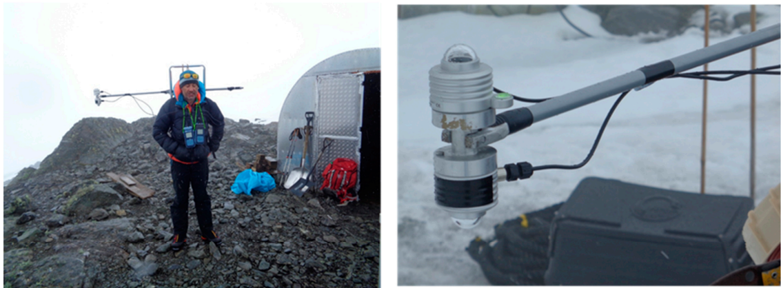
Figure 2. Portable albedometer and experimental set-up.
