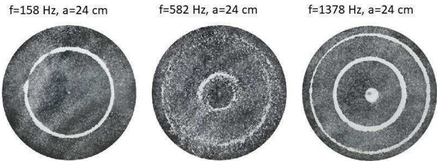
Figure 3. Nodal line patterns observed in the larger circular plate, a = 24 cm.
