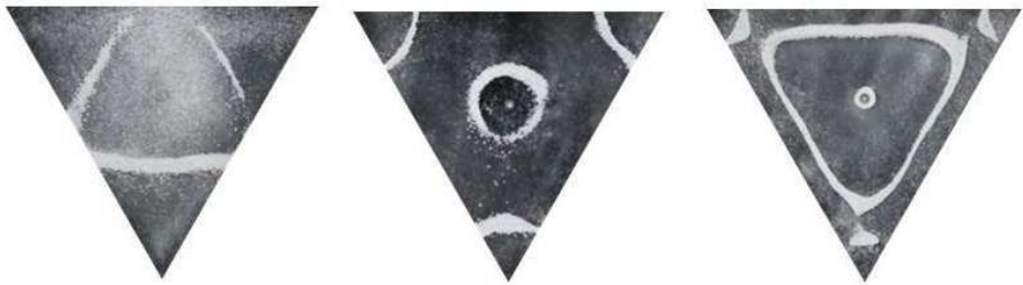
Figure 8. Nodal line patterns observed in the smaller triangle plate, a = 18\text{ cm} .
