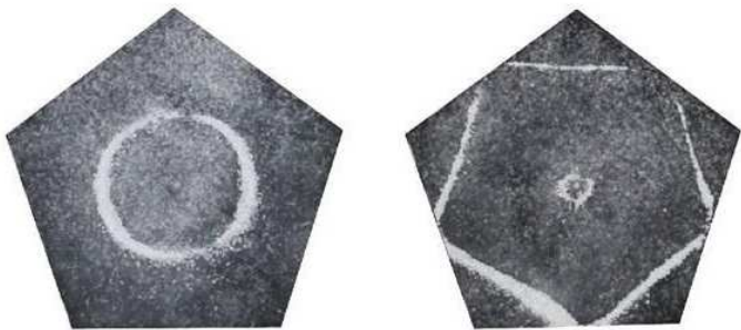
Figure 10. Nodal line patterns observed in the smaller pentagon plate, a = 9.5\text{ cm} .
