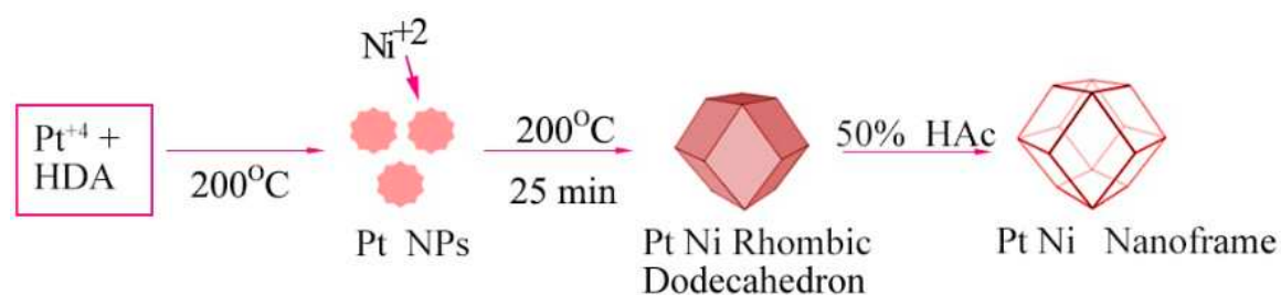
Figure 10. Schematic illustration for the synthesis of Pt-Ni dodecahedral nanoframe.
