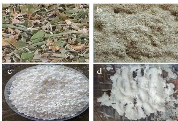
Figure 2. Physical appearance of (a) Chopped Typha augostifolia green leaf (b) Dried and crushed Typha augostifolia , (c) Isolated cellulose from Typha augostifolia and (d) Cellulose nanocrystals from Typha augostifolia .
