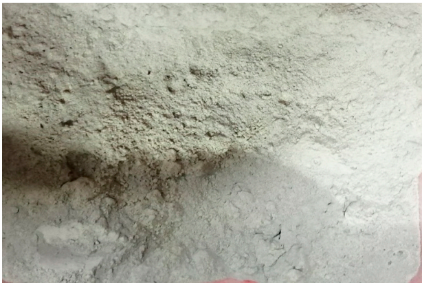
Figure 1. Silica fly ash used to futher tests.
