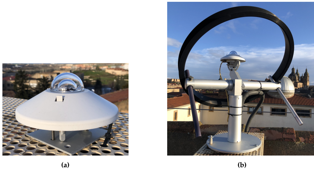
Figure 7. Measurement devices installed on the rooftop of the Trilingüe building of the Faculty of Sciences (40.96062 N, 5.67075 W) of the University of Salamanca (Spain): (a) Pyranometer Kipp & Zonen SMP10, (b) Pyranometer SMP10 with shadow ring model Kipp & Zonen CM 121.
