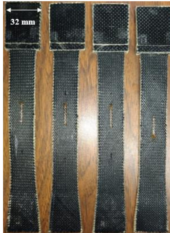
Figure 17. Condition of coupons after the tensile tests at [+45^\circ, -45^\circ]_s .
