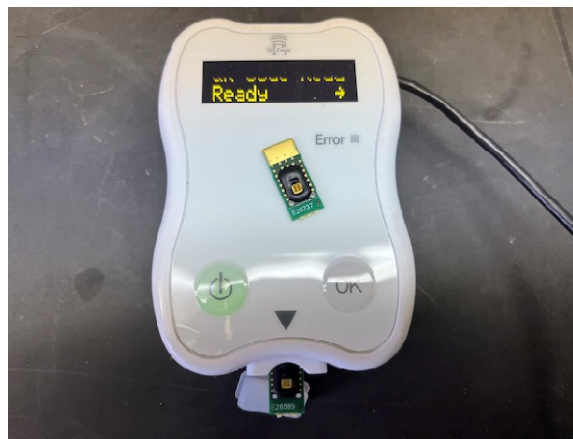
Figure 1. SH-SAW Biosensor System and gold-coated biosensor from TST Biomedical Electronics, (Taiwan). The sample reservoir is the black circle that surrounds the gold area that is visible in the middle of the biosensor.
