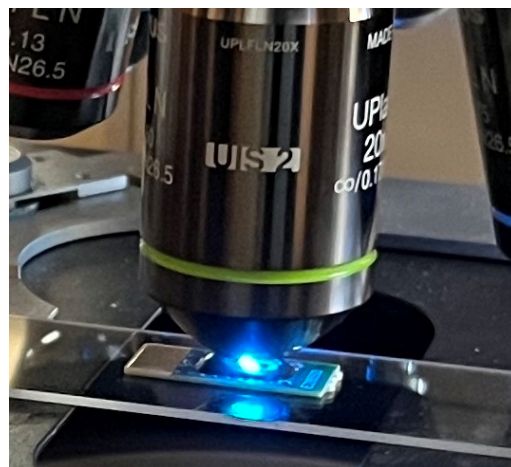
Figure 2. Photograph of the SH-SAW gold-coated biosensors with E. coli immobilized being imaged using epi-fluorescence microscopy.
