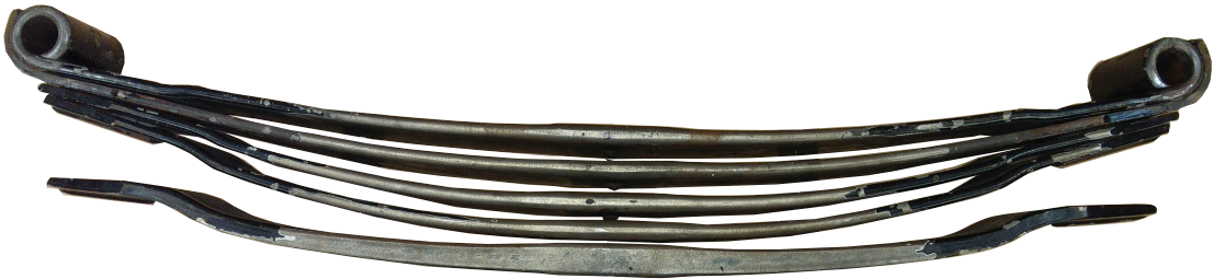
Figure 4. Leaf spring geometry before the assembling process.
