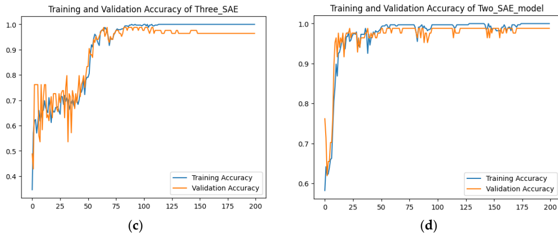
Figure 8. The accuracy results for data-class dataset detection. (a) CNN model, (b) LSTM model, (c) Proposed model (3-SAE), (d) Proposed model (2-SAE).
