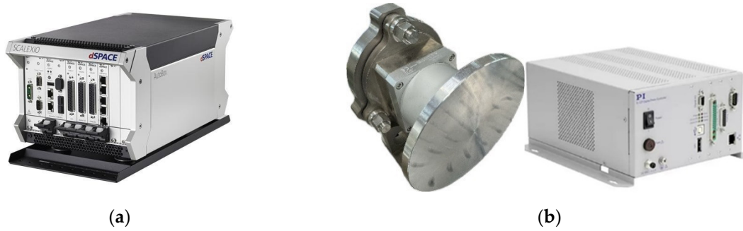
Figure 2. Experimental setup for fast steering mirror (FSM) control system: (a) Scalexio AutoBox (dSPACE), and (b) tip-tilt actuating platform (PI Ceramic GmbH).
