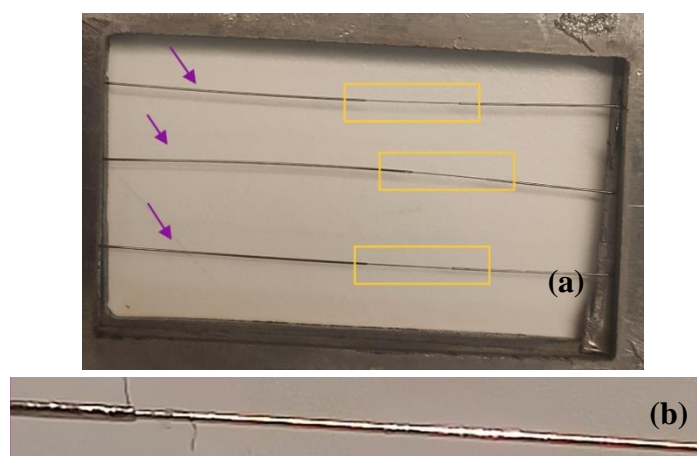
Figure 2. (a) Sputtering mask with 3 optical fibers with an FBG in the center of the fiber where the plastic cover has been removed (in the yellow boxes). Nickel sputtered optical fiber with a thickness of 100nm, (b) Optical fiber after nickel chemical deposition of 5\mu\text{m} thickness.
