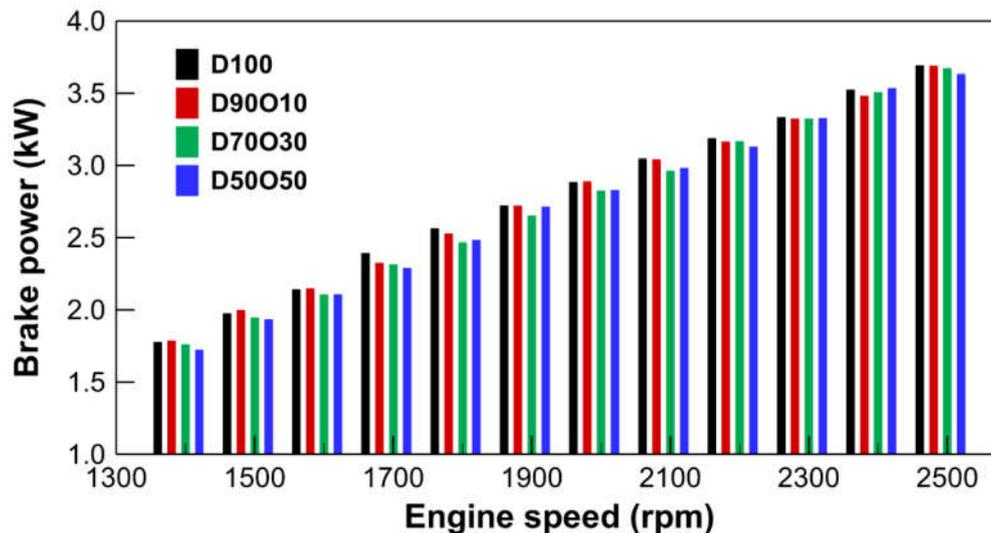
Figure 3. Comparison of brake power with engine speed for test fuels.
