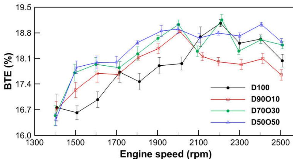
**Figure 4.** Comparison of brake thermal efficiency with engine speed for test fuels.
