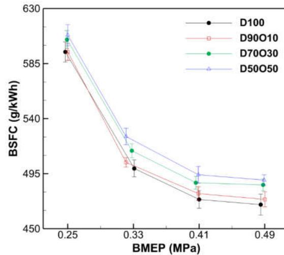
**Figure 7.** Comparison of brake specific fuel consumption with brake mean effective pressure at 1700 rpm.
