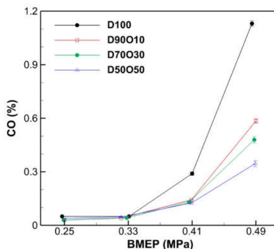
**Figure 9.** Comparison of CO emissions with brake mean effective pressure at 1700 rpm.
