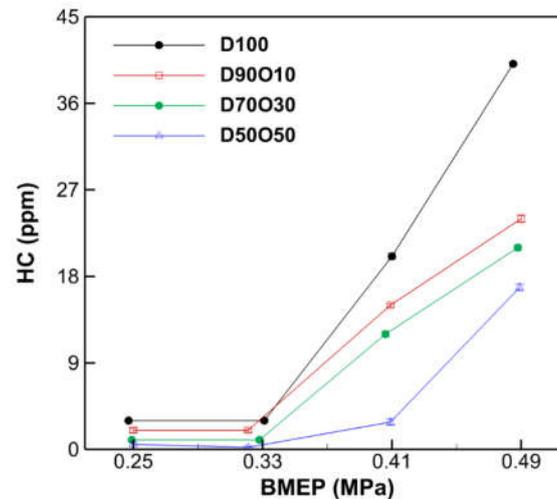
**Figure 10.** Comparison of HC emissions with brake mean effective pressure at 1700 rpm.
