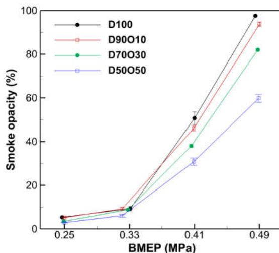
**Figure 11.** Comparison of smoke opacity with brake mean effective pressure at 1700 rpm.
