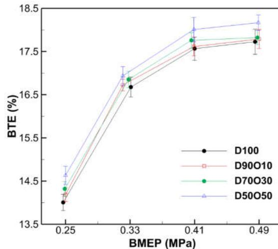
**Figure 6.** Comparison of brake thermal efficiency with brake mean effective pressure at 1700 rpm.
