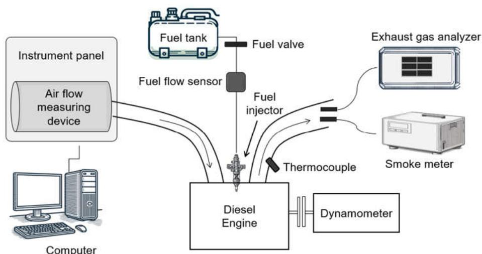
**Figure 1.** Schematic diagram of experimental apparatus.
