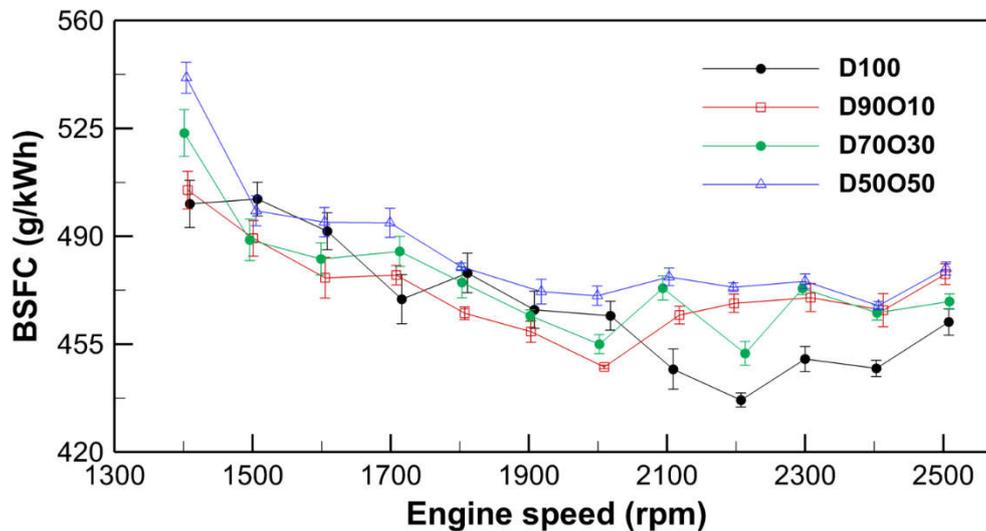
**Figure 5.** Comparison of brake specific fuel consumption with engine speed for test fuels.
