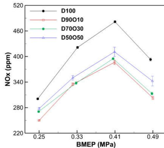
**Figure 8.** Comparison of NO<sub>x</sub> emissions with brake mean effective pressure at 1700 rpm.
