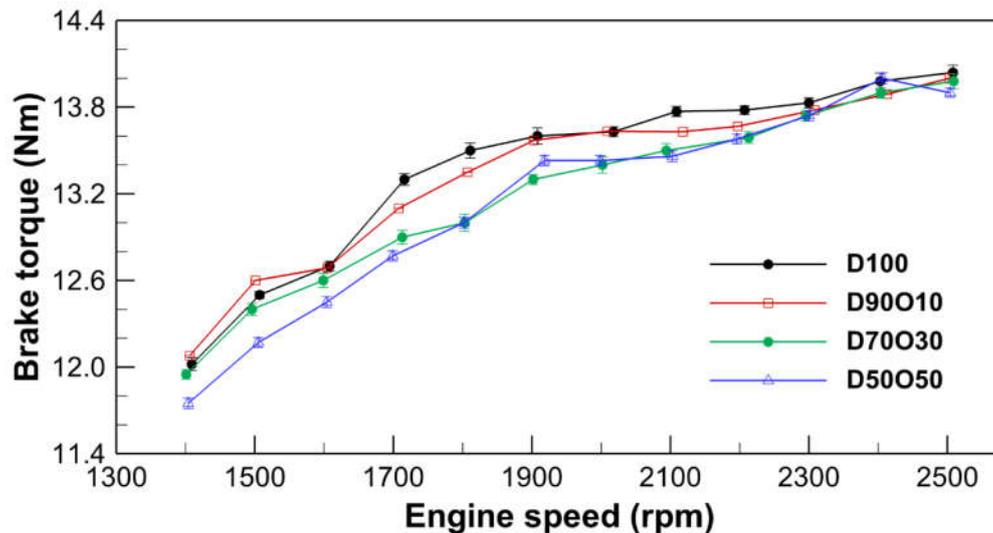
Figure 2. Comparison of brake torque with engine speed for test fuels.
