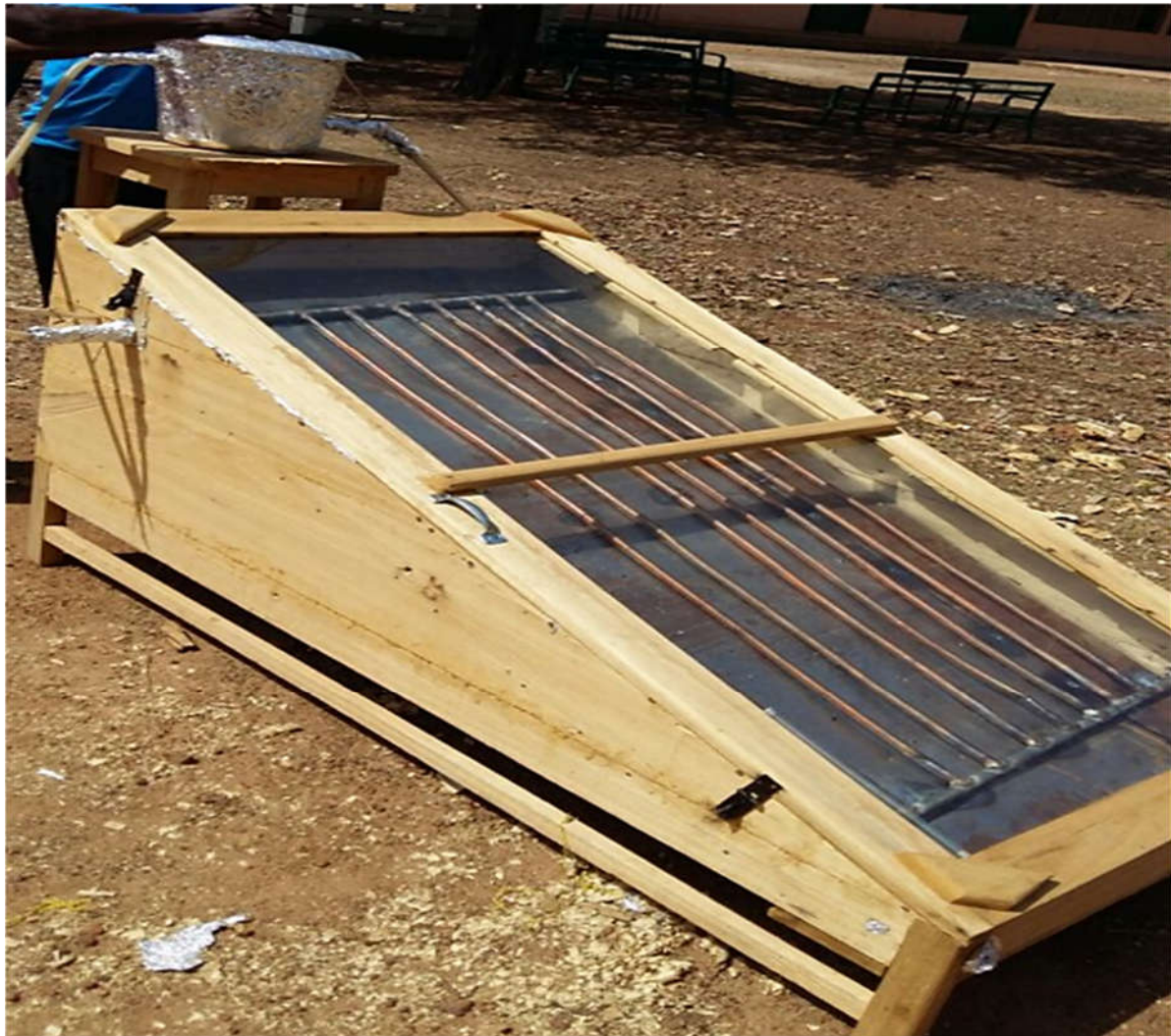
Figure 4. Complete diagram of the solar milk pasteurizer (Actual system).
