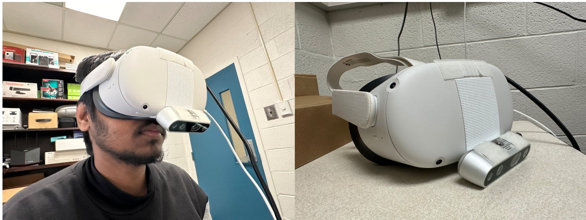
Figure 2. Setup for SmartVR Pointer with the camera mounted at the bottom of the Meta Quest 2 HMD.
