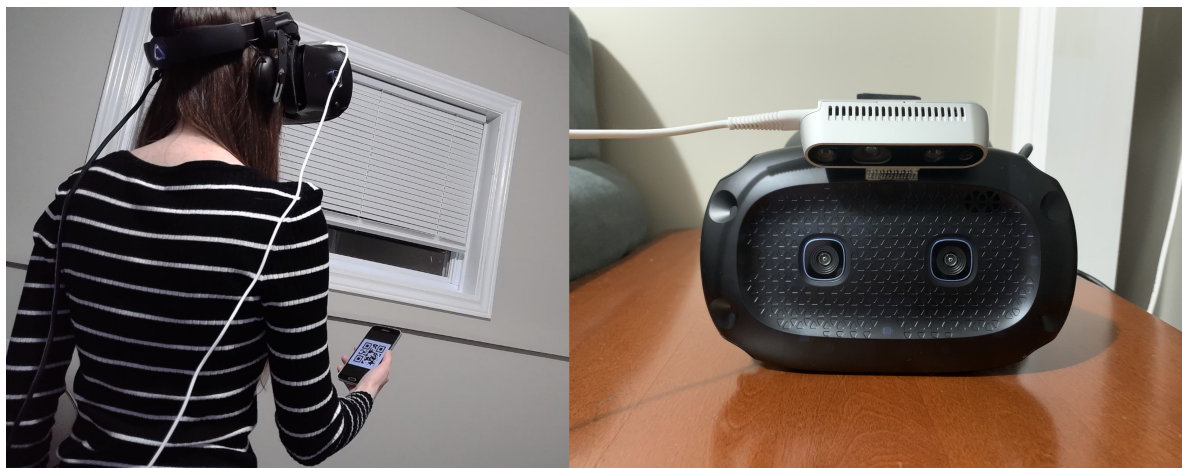
Figure 1. Setup for SmartVR Pointer with the camera mounted on top of the HTC Vive Cosmos Elite HMD.
