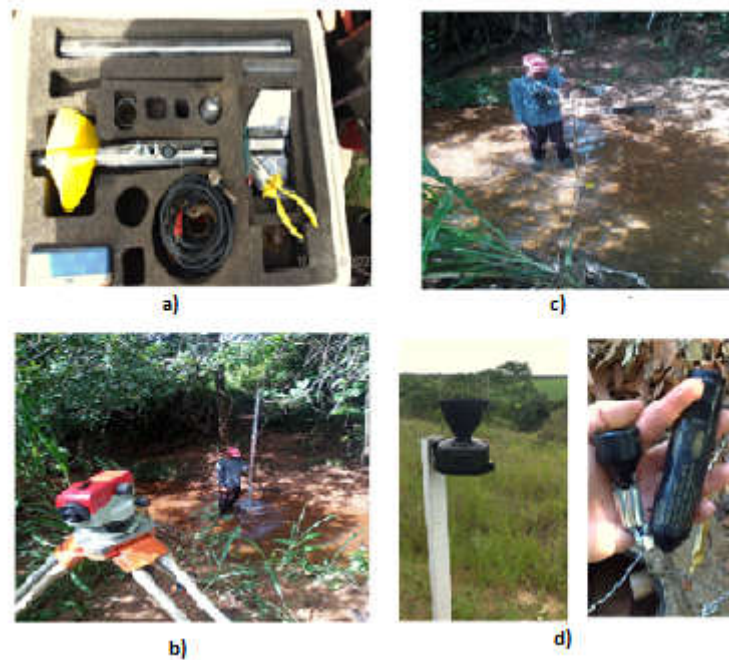
Figure 3. Equipment used in the monitoring of the sub-basin of the Pau de Caixeta stream. a) hydrometric windlass; b) river bathymetry; c) river flow measurement; d) pluviograph and linigraph.
