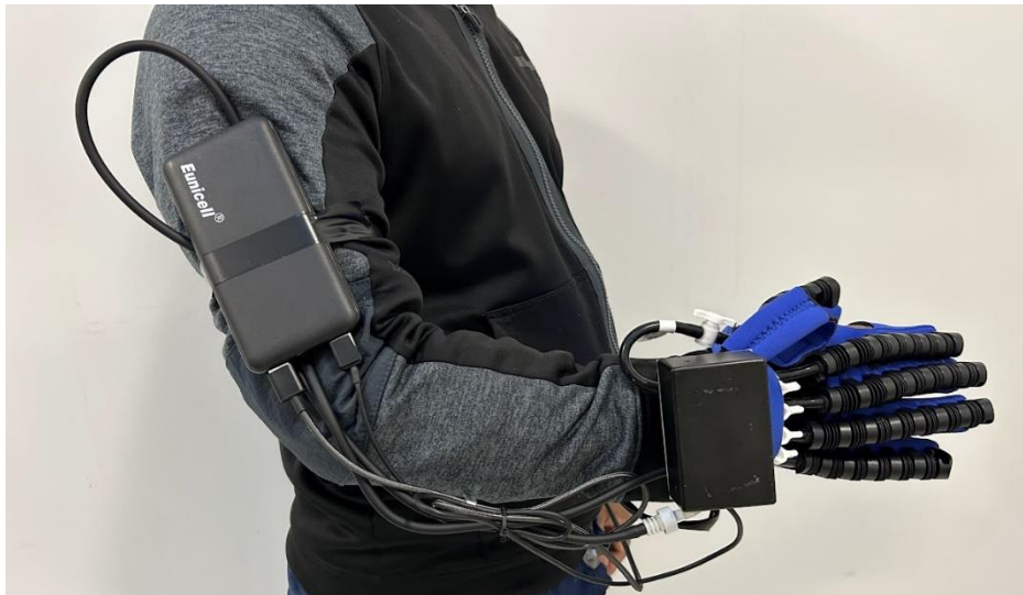
Figure 1. Prototype of AI cameras and sensors for hand exoskeleton.
