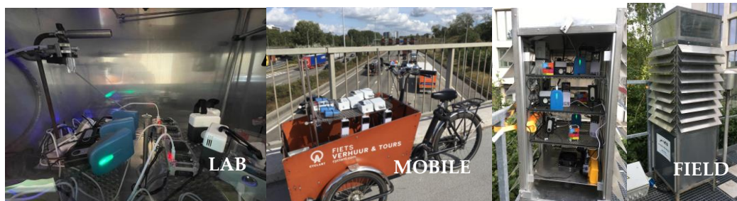
Figure 2. Pictures of the laboratory PM exposure chamber (left), mobile field test with cargo bike (middle) and field co-location (right) campaign at an urban background monitoring station.
