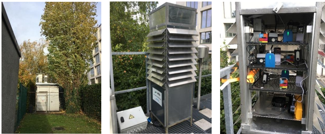
Figure 8. Location of the exposure shelter on top of R801 (left), detail of the exposure shelter (middle) and positioning of the sensor systems inside the shelter (right).
