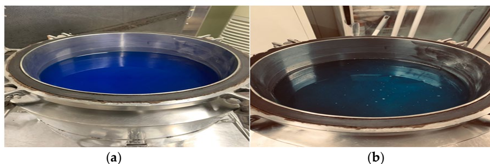
Figure 5. The Production of vanadium electrolyte (3.5 + ) using a 20-liter hydrothermal reactor: (a): vanadium (4 + ) in 20L hydrothermal reactor, (b): vanadium (3.5 + ) appearance.
