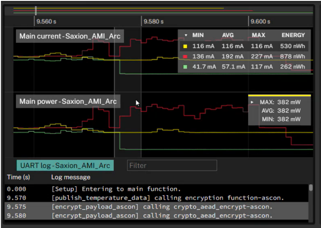
Figure 12. Power Analysis Read of LOLIN32 Lite ESP32 Using Otii-arch Device.
