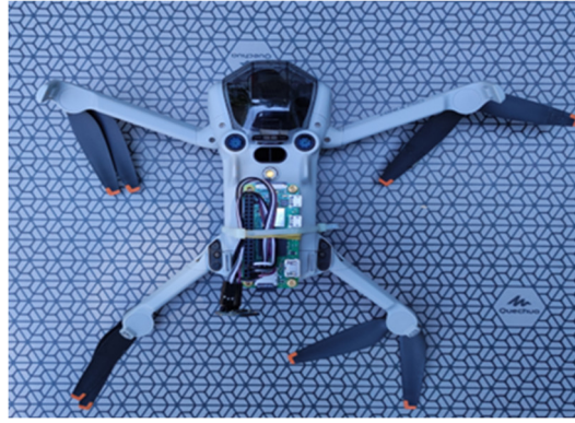
Figure 1. Equipping the DJI Mini 4 Pro drone with the Vishay VEML 6075 digital sensor.
