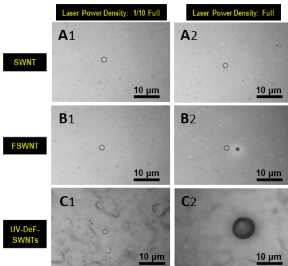
**Figure 5.** Microscope images of the Raman laser-irradiated sample areas: (A1, A2) pristine SWNTs, (B1, B2) untreated FSWNTs, and (C1, C2) crosslinked UV-DeF-SWNTs irradiated at 1/10 (Column 1) and full (Column 2) power density, respectively. Full power density: 2.9  $\text{kW}/\text{mm}^2$ .
