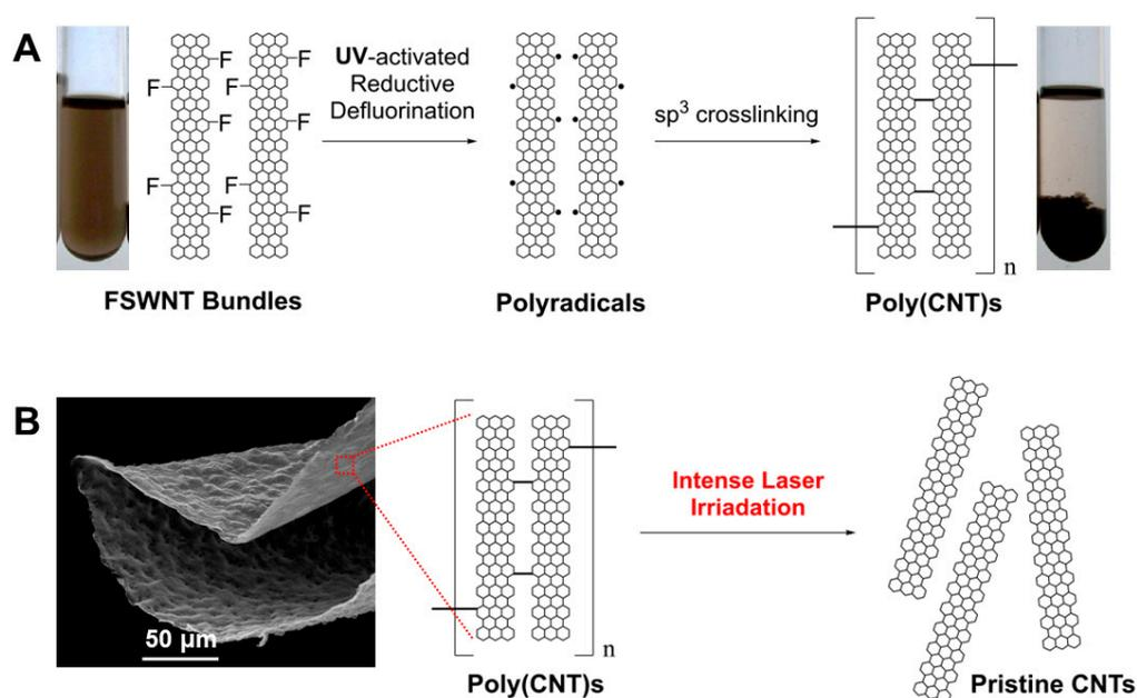
**Figure 1.** (A) Generation and recombination of free radicals in FSWNT bundles to form poly(CNT)s, as described in our previous work [23]; (B) Thermal stability of crosslinked CNTs, the primary focus of the current study.
