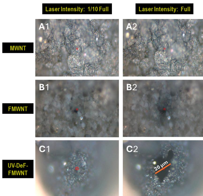
**Figure 7.** Microscope images of various MWNTs irradiated with a 532 nm Raman laser at 1/10 full power density (Left, Column 1) and full power density (Right, Column 2). (A) Pristine MWNTs, (B1) Untreated FMWNTs, and (C) UV-defluorinated MWNTs (UV-DeF-MWNTs).
