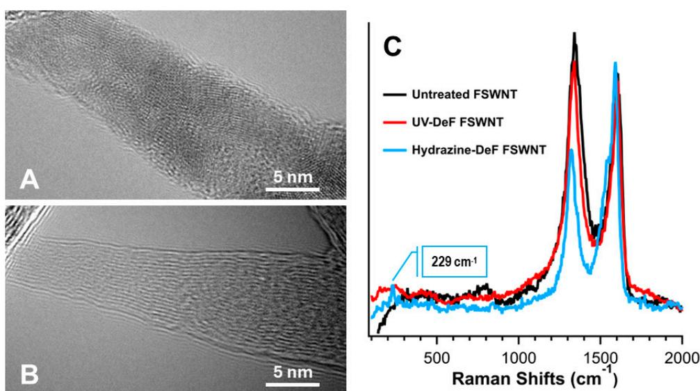
**Figure 2.** (A) TEM images of untreated fluorinated single-walled carbon nanotubes (FSWNTs) and (B) UV-crosslinked FSWNTs. (C) Raman spectra of untreated, UV-defluorinated, and hydrazine-defluorinated FSWNTs, recorded using a 532 nm laser wavelength with a power density of 2.9 kW/mm<sup>2</sup>.
