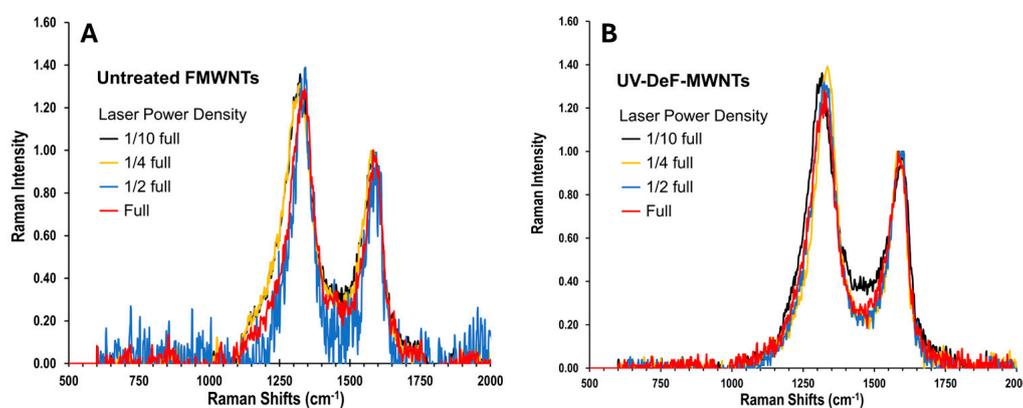
**Figure 6.** Raman spectra of (A) untreated FMWNTs and (B) UV-Defluorinated FMWNT (UV-DeF-MWNTs). Laser wavelength: 532 nm, with a full power density of 2.9kW/mm<sup>2</sup>.
