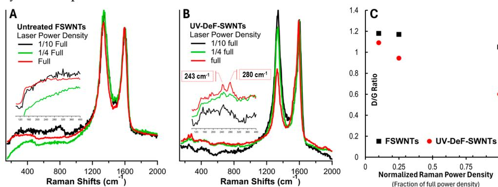
**Figure 3.** Raman spectra of (A) untreated FSWNTs and (B) UV-defluorinated crosslinked FSWNTs. (C) D/G ratio of untreated FSWNTs and UV-DeF-FSWNTs as a function of the fraction of full Raman laser power density. The Raman laser wavelength is  $532\text{ nm}$ , with a full laser power density of  $2.9\text{ kW/mm}^2$ . Insets in A and B show amplified RBM bands.
