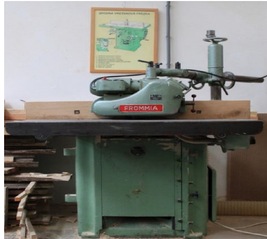
Figure 4. Lower spindle milling machine FVS and feeder mechanism Frommia ZMD 252/137.
