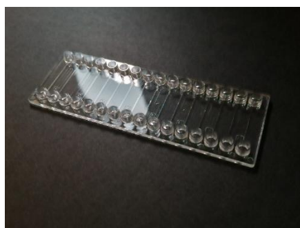
Figure 4. Example of a polymer transfer standard chip.
