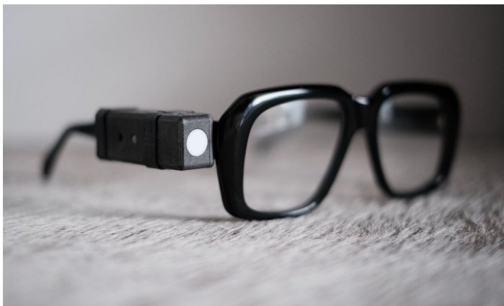
Figure 9. The wearable light dosimeter “lido” attached to a pair of glasses. The white circle is the diffuser. The small grey circle on the left is an indicator light that flashes green every 10 s (0.1 Hz) when recording.
