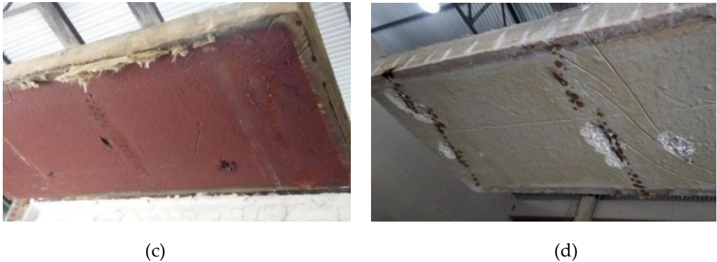
Figure 6. Top view of the concrete slabs during the fire exposure campaign (water pooling visible): (a) FNS-AAC slab, (b) OPC slab; (c) FNS-AAC slab and (d) OPC slab (limited spalling).
