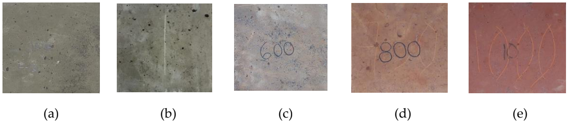
Figure 4. Color evolution as a function of temperature of exposure: 20 °C (a); 400 °C (b); 600 °C (c); 800 °C (e); and 1000 °C (d).
