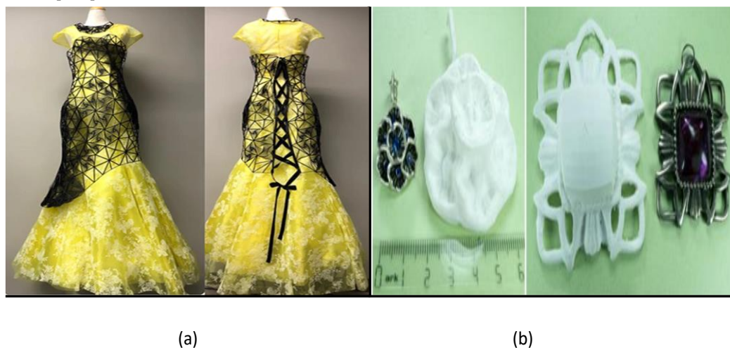
Figure 7. (a) FDM 3D printed dress and (b) Original and material extrusion printed view of jewellery. (Figure is reproduced from Ref. [133,134] with permission from Springer Nature).
