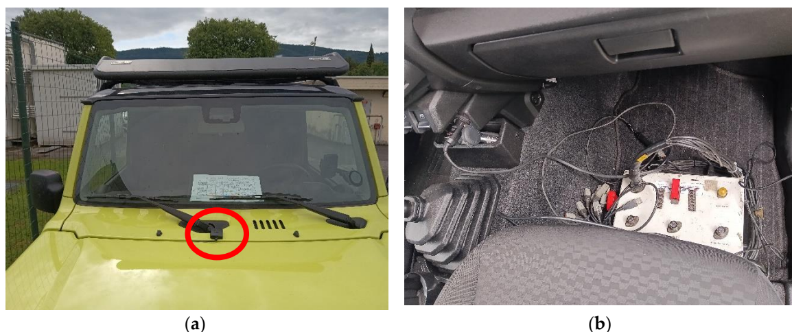
Figure 1. Location (a) of the GPS receiver (red circle), installed on the vehicle hood via magnetic connection, and (b) of the MoTeC ADL2 data acquisition unit, on the passenger mat, inside a protective box.
