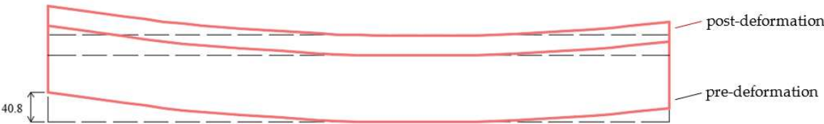
Figure 8. S Schematic Diagram of Lateral Deformation for Traditional Hinged Widened Bridges (units: mm).
