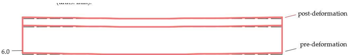
Figure 8. S Schematic Diagram of Lateral Deformation for Traditional Hinged Widened Bridges (units: mm).
