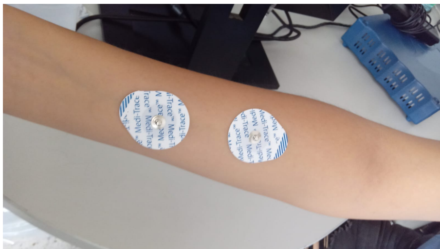
Figure 1. Two electrodes were placed on the forearm; a third electrode was placed near the elbow (not visible in the image).
