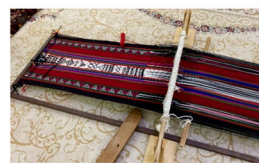
Pl. 3: The enhanced simple loom, noting the iron legs below (Photographed by the Researchers, 2024)
