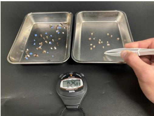
Figure 5. Photograph of the visual sorting process, showing the manual separation of particles.
