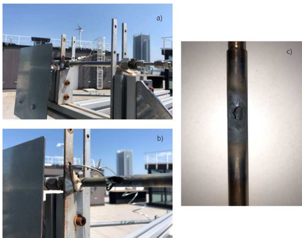
Figure 9. Experimental activity for the metal alloys used a: Inconel 740H; b: alloy 625; c: Haynes 230.
